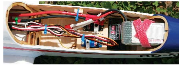
The forward fuselage offers plenty of room for installing the radio. I extended the ESC's battery leads to reach the battery mounted in the nose. A few wire ties help neaten up the overall installation.
